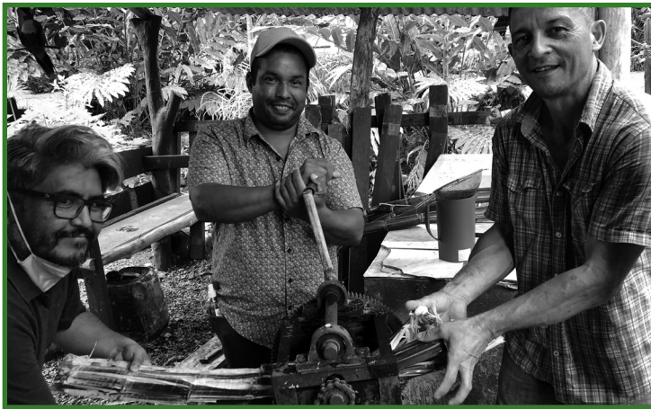
Jose Araya, farm manager of SIFAT's Central American Training Center in Costa Rica, demonstrates an appropriate technology sugar cane press made of old car parts to Oscar Fereira and Josue Matute, director of the Agroecology Center at UNA in Honduras.
